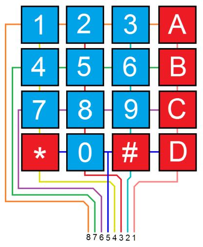
Figure 1: Matrix Keypad Connections
